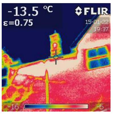
In this thermal image maximum heat loss is shown by white/red colour.
